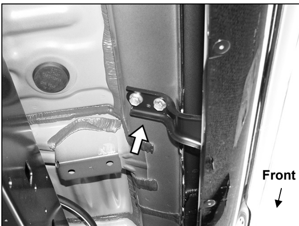
(Fig 3) Remove (2) hex bolts from passenger/right center mounting location (arrow)
