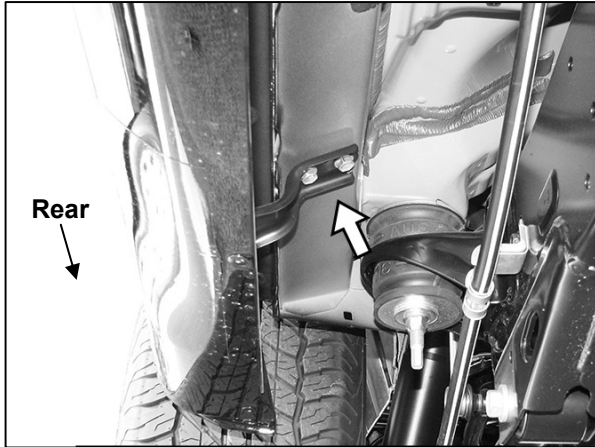
(Fig 5) Remove (2) hex bolts from passenger/right rear mounting location (arrow)
