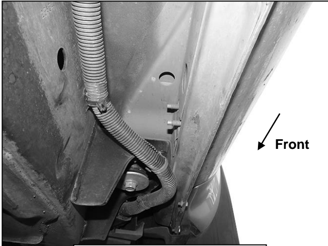
(Fig 1) Passenger/Right side front mounting location
