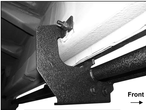
(Fig 31) Driver/left #3 Bracket with Running Board
