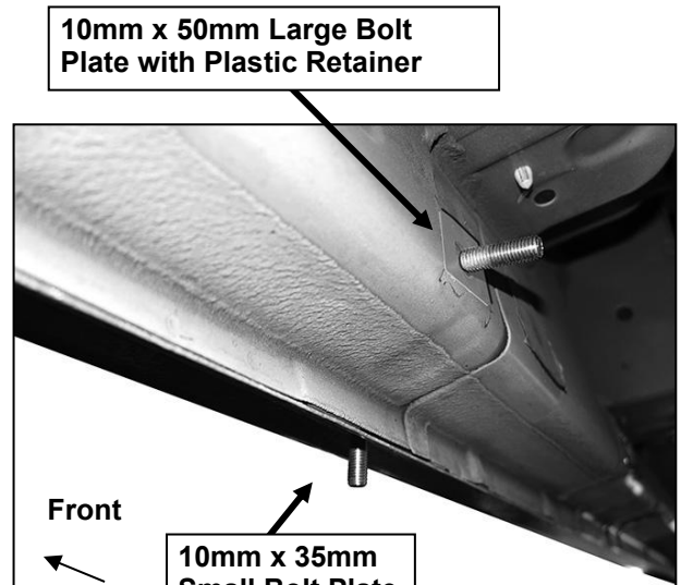
(Fig 5) Passenger/right #2 mounting location
