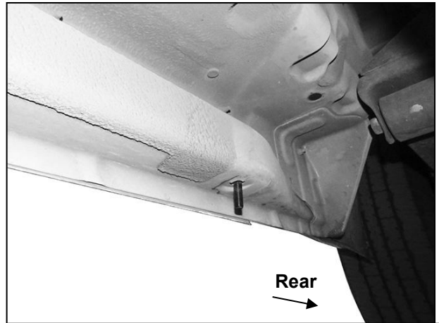
(Fig 10) Passenger/right rear mounting location
