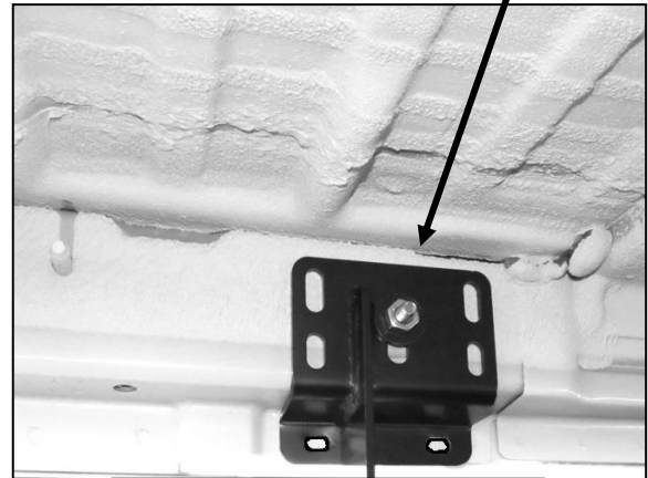
(Fig 7) Push all Brackets up tight against body panel
