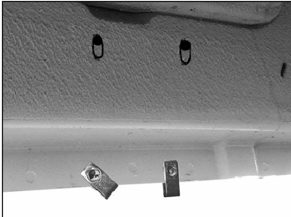
(Fig 23) Model without existing holes, drill 3/8" holes at marked locations for U-Bolts, 5/16" through pinch weld for Clip Nuts.
