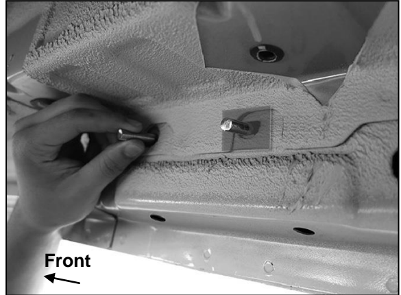
(Fig 24) Insert 8mm U-Bolt into and out holes in body panel (see Fig 22 & 23). Thread 8mm Plastic Retainers onto U-Bolt to help hold in place (retainer use is not mandatory for installation)
