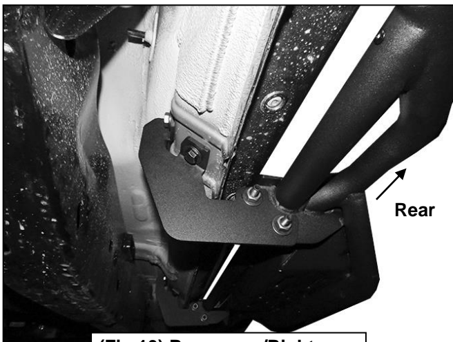
(Fig 10) Passenger/Right Rear Running Board installed
