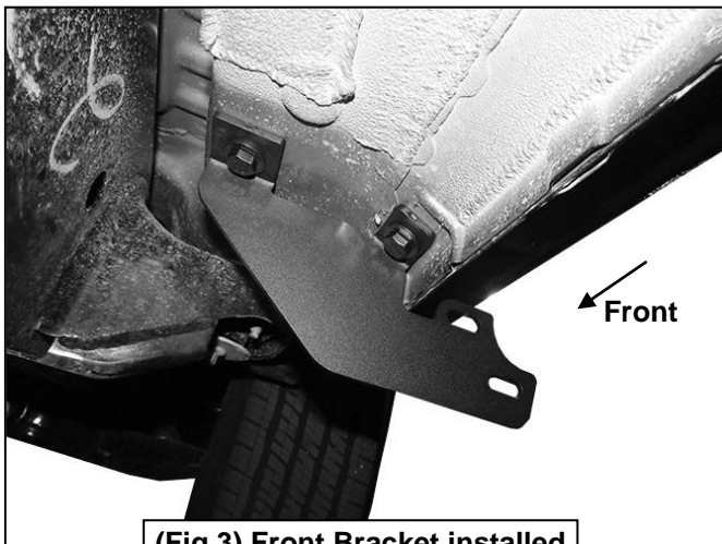
(Fig 3) Front Bracket installed
