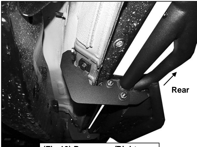
(Fig 10) Passenger/Right Rear Running Board installed
