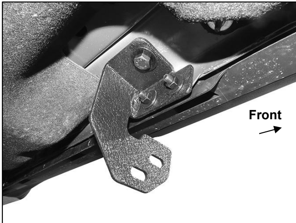
(Fig 7) Driver/left center Bracket installed
