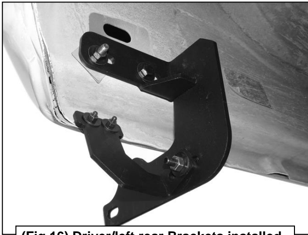
(Fig 16) Driver/left rear Brackets installed
