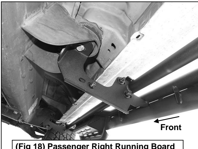
(Fig 18) Passenger Right Running Board attached to the Center Mounting Bracket
