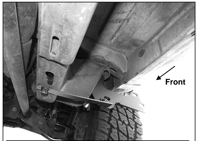
(Fig 7) Passenger/Right Front Support Bracket attached to the frame and Mounting Bracket
