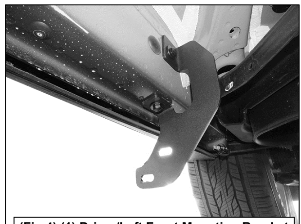
(Fig 4) (1) Driver/Left Front Mounting Bracket attached to the Driver/Left front location
