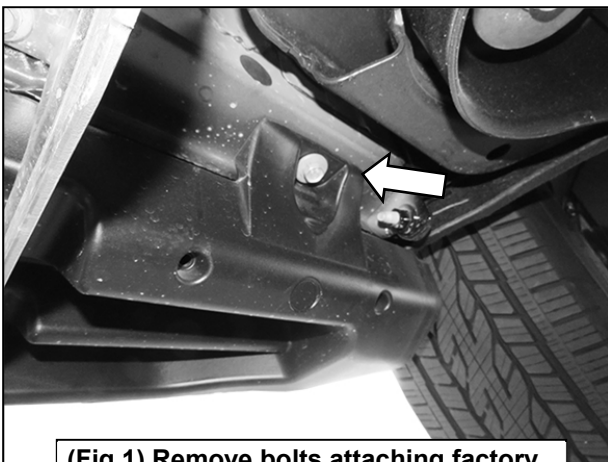
(Fig 1) Remove bolts attaching factory Running Board to Rocker Panel
