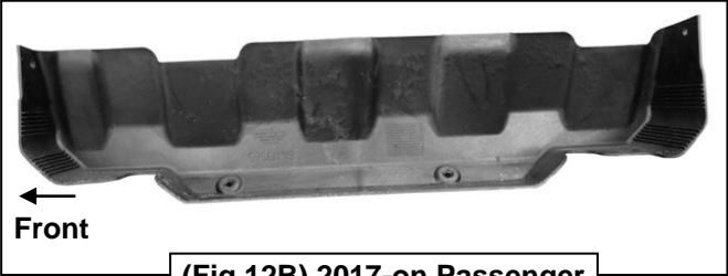
(Fig 12B) 2017-on Passenger side DEF cover removed
