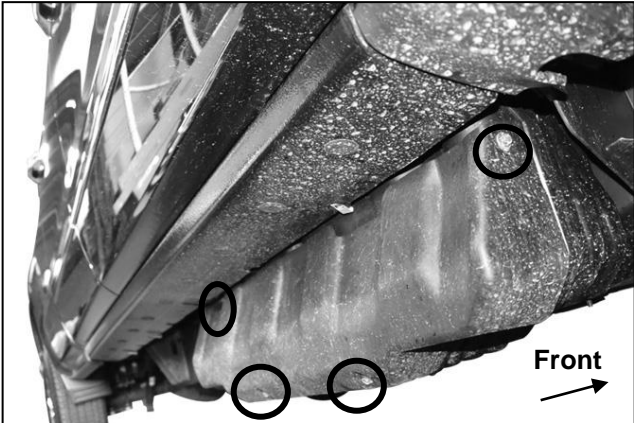
(Fig 12A) 2017 Passenger side pictured with DEF plastic tank cover. Remove (4) hex bolts to remove plastic cover
