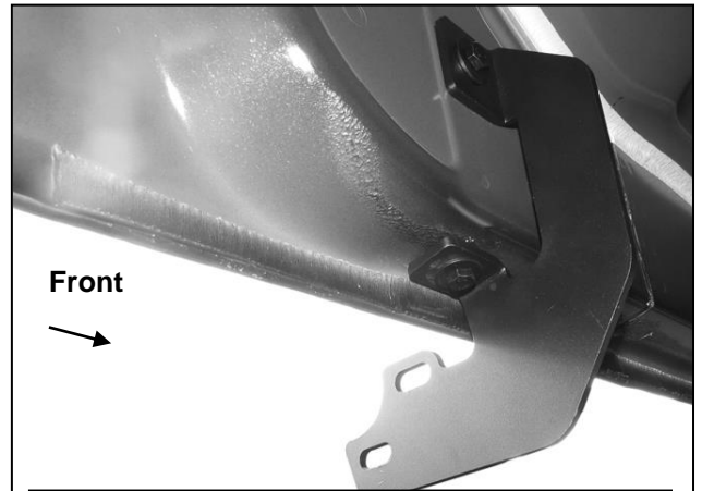
(Fig 10) Driver/left side rear Bracket installed
