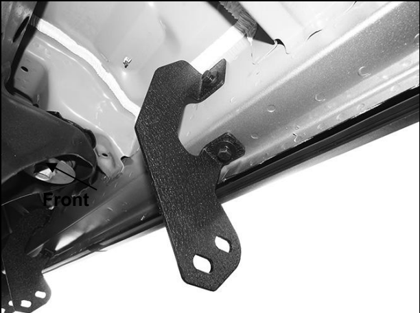
(Fig 5) Driver/left #2 Mounting Bracket installed
