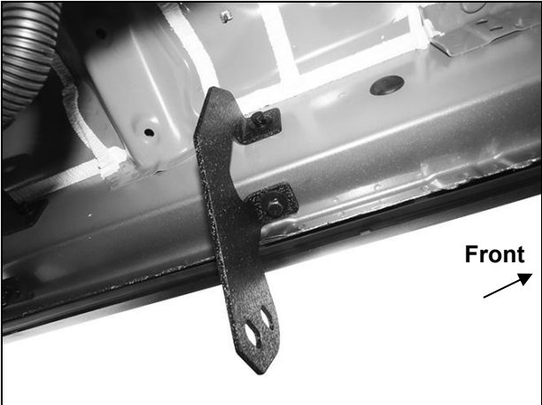
(Fig 7) Driver/left #3 Mounting Bracket installed
