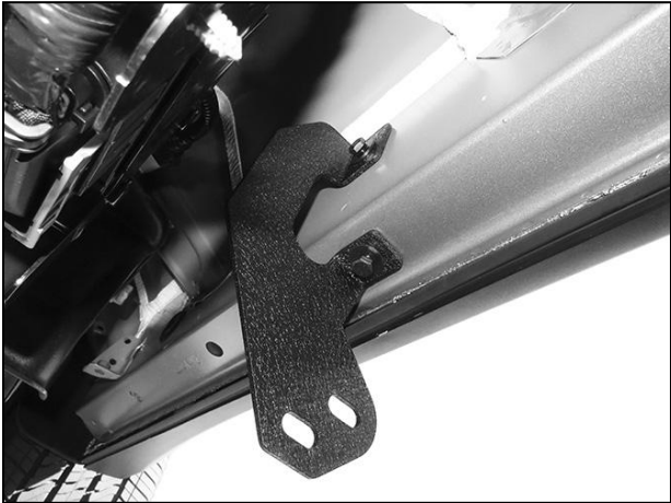
(Fig 8) Driver/left rear Mounting Bracket installed
