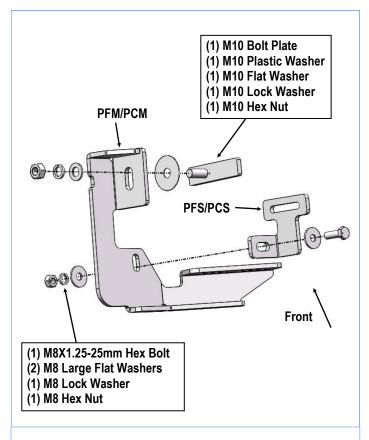
(Fig 3) Passenger Front Mounting Bracket (PFM/PCM) and Passenger Front Support Bracket (PFS/PCS) Installation
