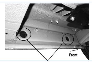
(Fig 12) Driver Side Front & Rear Mounting Locations
