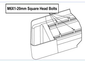
(Fig 8) Slip M6X1-20mm Square Head Bolts Into The Bottom Channels
