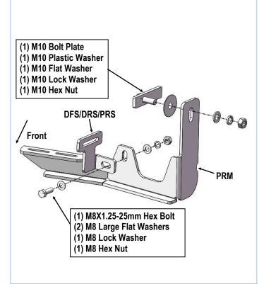
(Fig 6) Passenger Rear Mounting Bracket (PRM) and Passenger Rear Support Bracket (DFS/DRS/PRS) Installation
