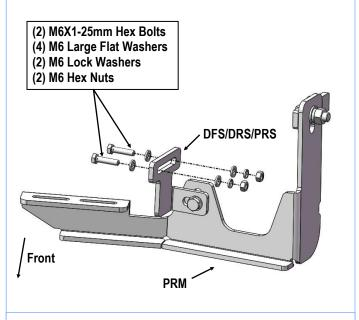
(Fig 11) Attach Support Bracket To Pinch Weld
