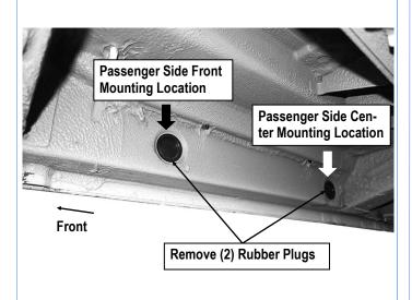
(Fig 1) Passenger Side Front & Center Mounting Locations
