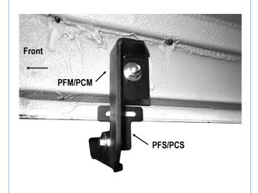
(Fig 4) Passenger Front Brackets Installed
