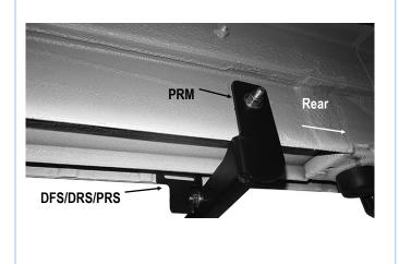
(Fig 7) Passenger Rear Bracket Installed
