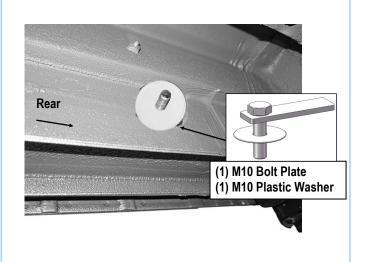
(Fig 5) Passenger Side Rear Mounting Location
