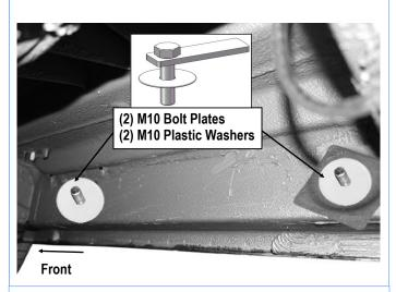
(Fig 2) M10 Bolt Plate Installed (On Passenger Side Front & Center Mounting Location)
