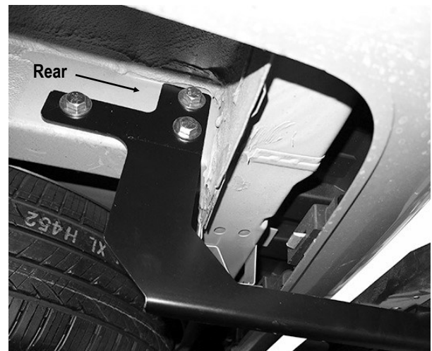
(Fig 3) Driver Side Mounting Brackets Installed
