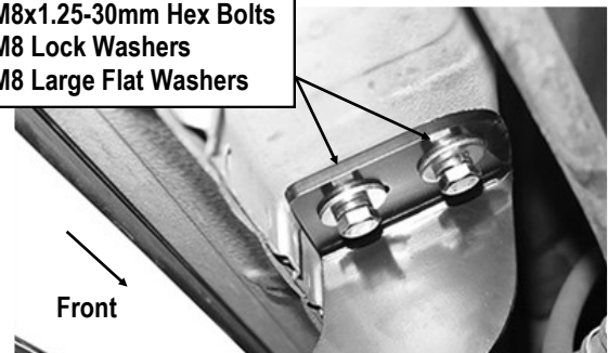
(Fig 7) Driver Center Mounting Bracket Installed
