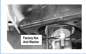
(Fig 2) Driver Rear Mounting Bracket Installation
