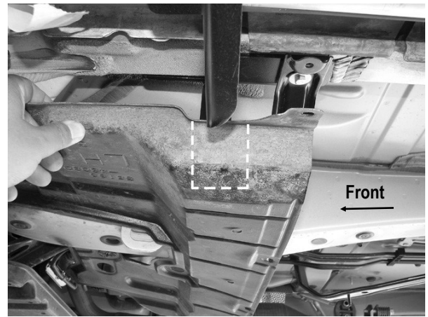
(Fig 19B) Hold Plastic Cover Up In Position To Determine Area To Cut From Cover. Driver Side Front Cover Pictured
