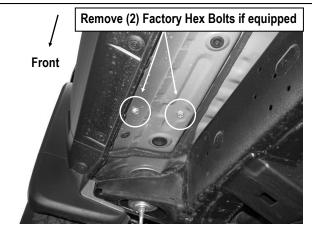
(Fig 1) Driver Side Front Mounting Location
