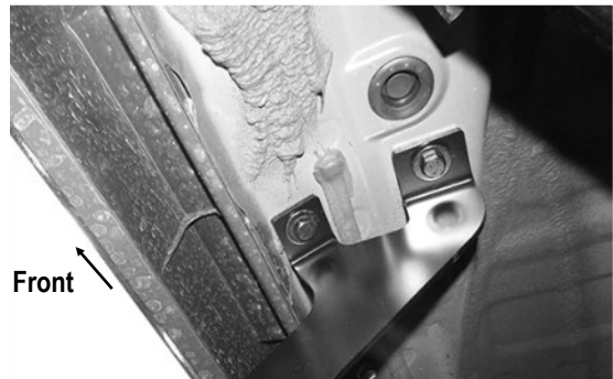
(Fig 3) Passenger Front Mounting Brackets Installed
