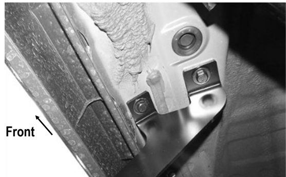
(Fig 3) Passenger Front Mounting Brackets Installed
