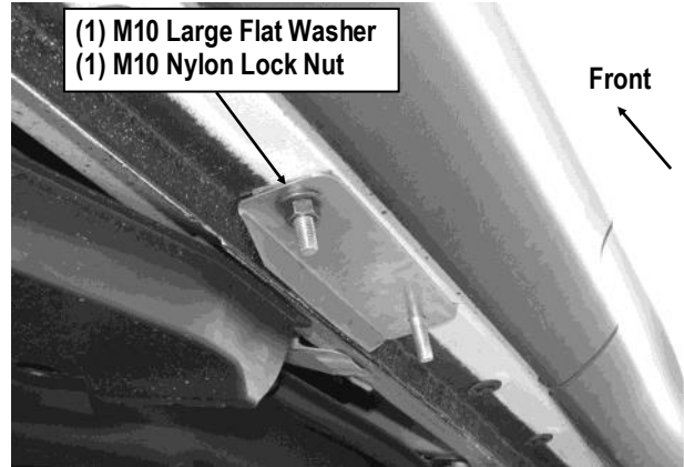
(Fig 9) Locking Plate (DCS1) Installation (Driver Side Center Mounting Location)
