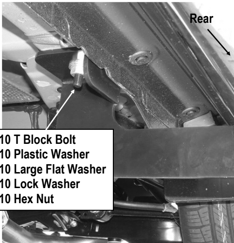
(Fig 9) Driver Side Rear Mounting Bracket Installation
