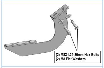
(Fig 4) Driver Center & Rear Mounting Bracket Installation
