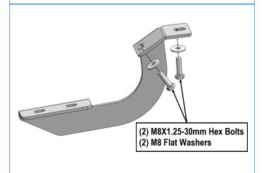
(Fig 2) Driver Front Mounting Bracket Installation
