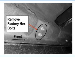
(Fig 3) Driver Side Center & Rear Mounting Location
