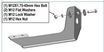
(Fig 6) Driver Rear Mounting Bracket (DRM) Installation
