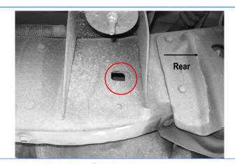
(Fig 5) Driver Side Rear Mounting Location
