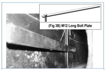
(Fig 3A) Inside View Of M10 Long Bolt Plate Installed (In Driver Side Frame Channel)
