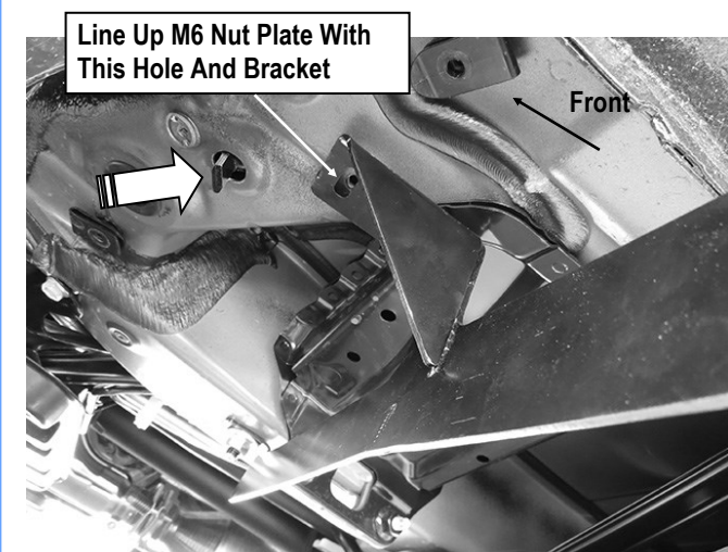
(Fig 5) Insert Nut Plate Into Factory Hole
