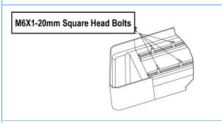
(Fig 4) Slip M6X1-20mm Square Head Bolts Into The Bottom Channels
