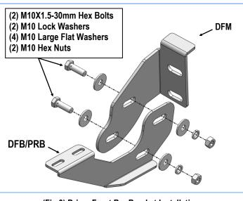
(Fig 3) Driver Front Bar Bracket Installation
