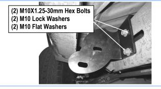
(Fig 2) Driver Front Mounting Bracket (DFM) Installed
