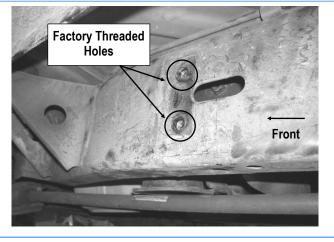
(Fig 1) Driver Side Front Mounting Location
