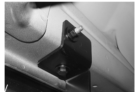
(Fig. 10) Driver Center Mounting Bracket Installed
