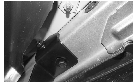
(Fig. 8) Driver Front Mounting Bracket Installed
