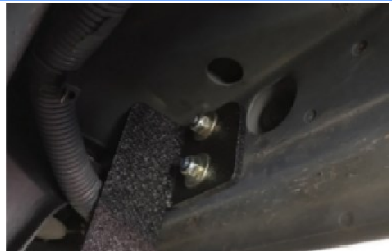
(Fig 3) Driver Side Front Mounting Bracket Installed
