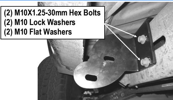
(Fig 2) Driver Front Mounting Bracket (DFM) Installed
