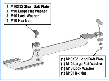
(Fig 2) Passenger Front Mounting Bracket Installation
