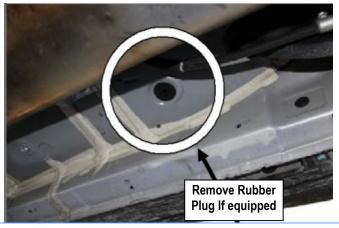
(Fig 3) Passenger Rear Mounting Bracket Installation
