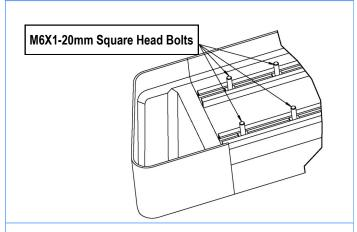
(Fig 8) Slip M6X1-20mm Square Head Bolts Into The Bottom
