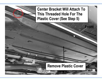
(Fig 1) Passenger Side Front Mounting Location Pictured
