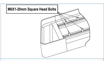
(Fig 12) Slip M6X1-20mm Square Head Bolts Into The Bottom Channels
