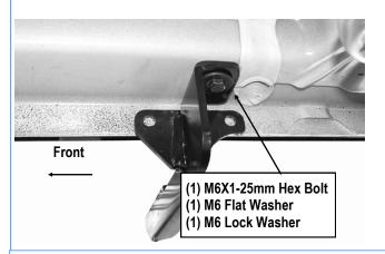
(Fig 7) Passenger Side Center Mounting Bracket Installation
