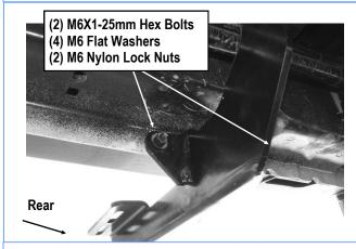
(Fig 16) Driver Side Rear Bracket Installation
