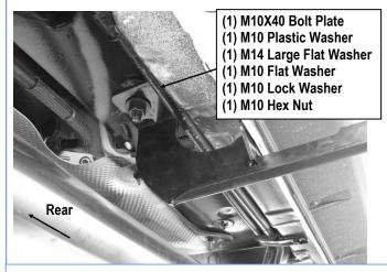
(Fig 11) Passenger Side Rear Mounting Bracket Installation
