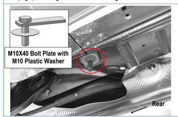
(Fig 9) Insert (1) M10X40 Bolt Plate
