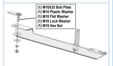
(Fig 5) Passenger Side Front Mounting Bracket Installation
