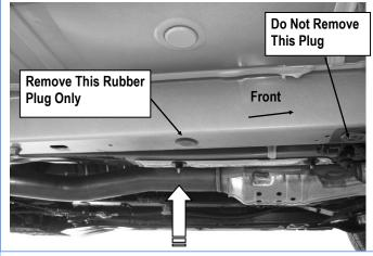
(Fig 2) Passenger Side Front Mounting Location Pictured
