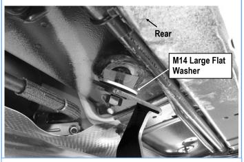
(Fig 10) Insert M14 Large Flat Washer Between The Bracket And The Body Panel
