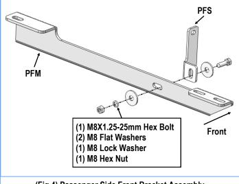
(Fig 4) Passenger Side Front Bracket Assembly
