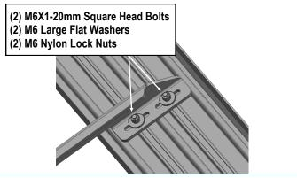
(Fig 13) Running Board Installed Onto Mounting Bracket
