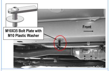
(Fig 3) Insert (1) M10X35 Bolt Plate with (1) M10 Plastic Washer
