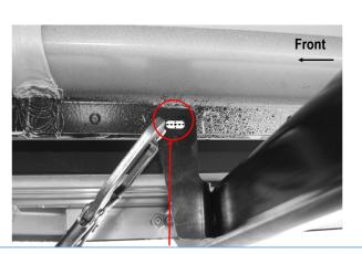
(Fig 14) Marking And Drilling Holes (Passenger Side Front Mounting Bracket )
