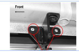
(Fig 15) Marking And Drilling Holes (Passenger Side Center Mounting Bracket )
