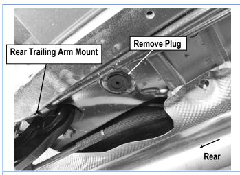
(Fig 8) Passenger Side Rear Mounting Location Pictured
