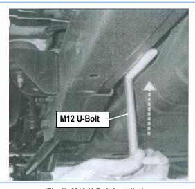
(Fig 1) M12 U-Bolt Installation
