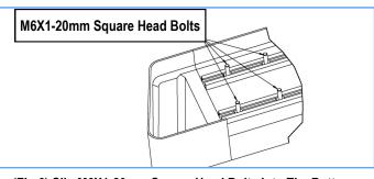
(Fig 6) Slip M6X1-20mm Square Head Bolts Into The Bottom Channels
