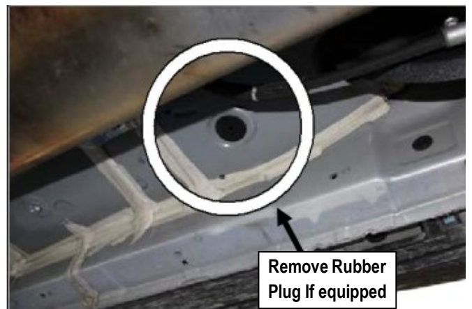
(Fig 3) Passenger Rear Mounting Bracket Installation
