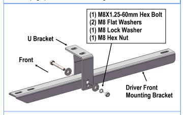
(Fig 8) Driver Front Mounting Bracket Installed
