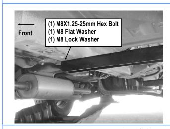
(Fig 7) Driver Front Mounting Bracket Installed
