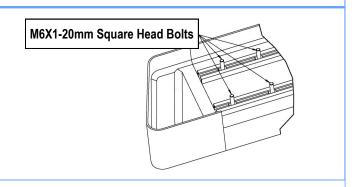
(Fig 12) Slip M6X1-20mm Square Head Bolts Into The Bottom Channels
