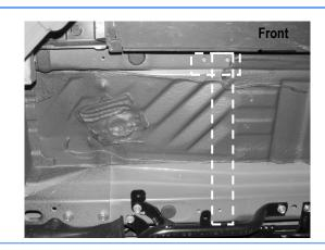
(Fig 5) Dashed Line Represents Driver Side Front Mounting Location For Bracket Assembly
