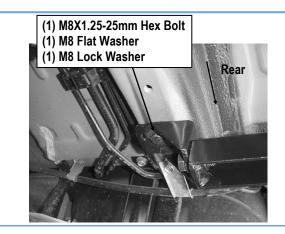
(Fig 10) Driver Rear Support Bracket Installed
