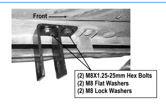
(Fig 6) Drive Front U Bracket Located
