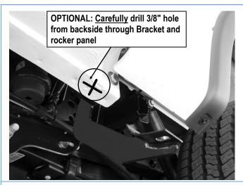
(Fig 11) Driver Rear Mounting Bracket Installed
