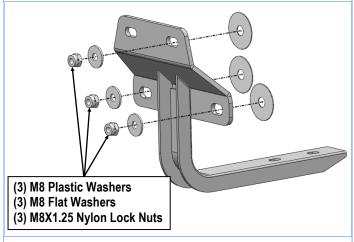
(Fig 6) Driver Front Mounting Bracket Installation
