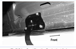
(Fig 7) Driver Front Mounting Bracket Installed
