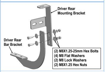
(Fig 14) Driver Rear Mounting Bracket Bar Bracket Assembly
