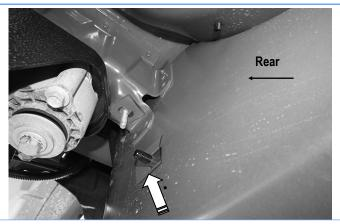
(Fig 13) Insert M10X40 Bolt Plate W/Plastic Washer into square hole. Thread another Plastic Washer onto Bolt Plate
