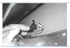
(Fig 5) File The M10 Clip Nut (On Center & Rear Mounting Locations)
