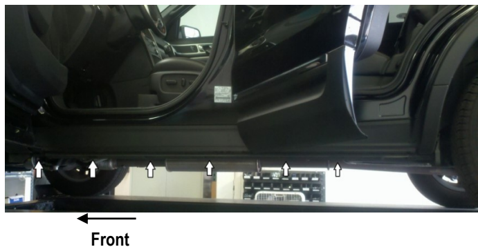
(Fig 3) Release Plastic Retainers Along The Body Panel
