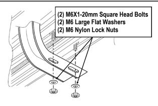
(Fig 8) Running Board Installed Onto Mounting Bracket
