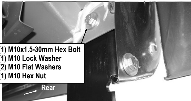
(Fig 7) Passenger Rear Mounting Bracket Installation
