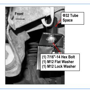
(Fig 4) Passenger Front Mounting Bracket Installation
