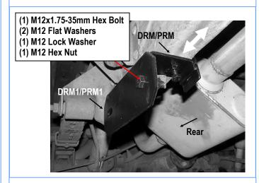
(Fig 6) Passenger Rear Mounting Bracket 1 Installation
