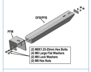
(Fig 3) Passenger Side Front Brackets Assembly
