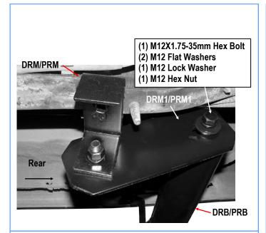
(Fig 7) Passenger Rear Bar Bracket Installation
