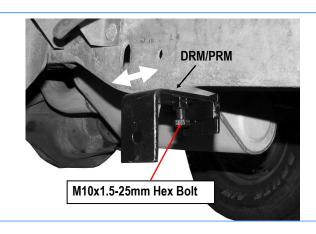
(Fig 5) Passenger Rear Mounting Bracket (DRM/PRM) Installation
