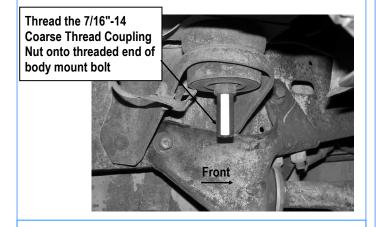
(Fig 2) 7/16"-14 Coarse Thread Coupling Nut Installation
