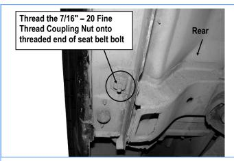
(Fig 8) Thread The 7/16" – 20 Fine Thread Coupling Nut Onto Threaded End Of Seat Belt Bolt
