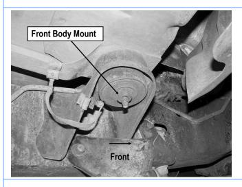
(Fig 1) Passenger Side Front Mounting Location
