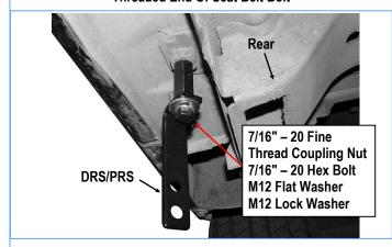
(Fig 9) Passenger Rear Support Bracket Installation
