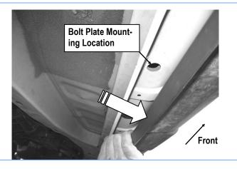
(Fig 2) Driver Side Front Mounting Location (Remove 3 Plastic Clips and pull out the trim panel)
