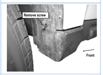
(Fig 1) Remove Screw from the front fender
