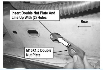
(Fig 9) M10X1.5 Double Nut Plate Installation
