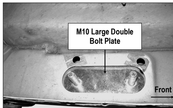
(Fig 3) M10 Large Double Bolt Plate Installed (On Driver Side Front Mounting Location)
