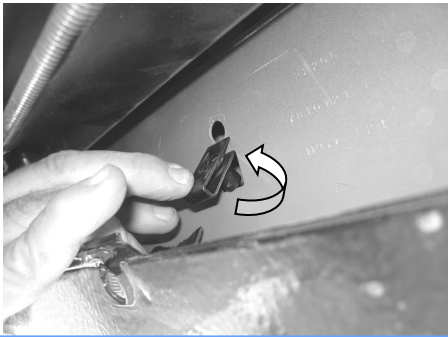
(Fig 5) File The M10 Clip Nut (On Center & Rear Mounting Locations)
