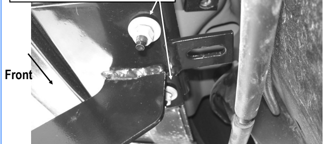
(Fig 2) Driver Front Mounting Bracket Installation
