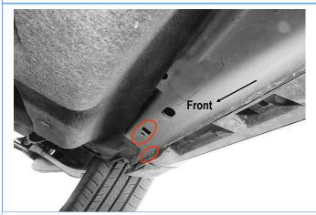
(Fig 1) Passenger Side Front Mounting Location
