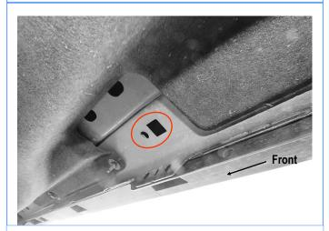
(Fig 5) Passenger Side Center Mounting Location
