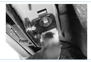
(Fig 4) Passenger Front Mounting Bracket Installation
