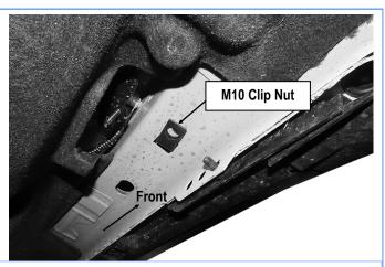
(Fig 2) Attach The M10 Clip Nut
