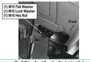
(Fig 2) Driver Front Mounting Bracket Installed
