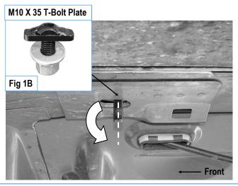
(Fig 1A) M10X35 T-Bolt Plate Installation
